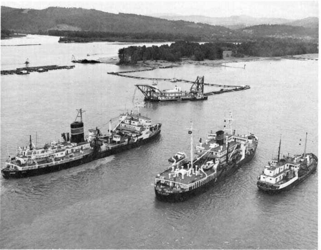
Mt. St. Helens Clean-up. The 18 May 1980 eruption of Mt. St. Helens sent massive amounts of mud and debris into the Toutle, Cowlitz, and Lower Columbia Rivers. Pictured are the Corps of Engineers hopper dredges BIDDLE, HARDING and PACIFIC with the Port of Portland pipeline dredge OREGON working to remove an estimated 14 million cubic yards of debris to restore the navigation channel depth to the Columbia River near Longview, Washington. Other dredges were working upstream on the Cowlitz River to restore its flow carrying capability. Mud and ash flows reduced the bankfull flow of the Cowlitz River at Castle Rock from 70,000 cfs to 7,000 cfs. The dredging efforts directed by the Corps of Engineers are expected to increase the bankfull capacity to 50,000 cfs.
