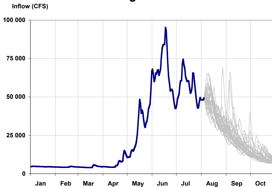
Figure 1 Series of synthetic hydrographs produced using the ESP forecasting procedure. Forecast date is 01 August in the example
